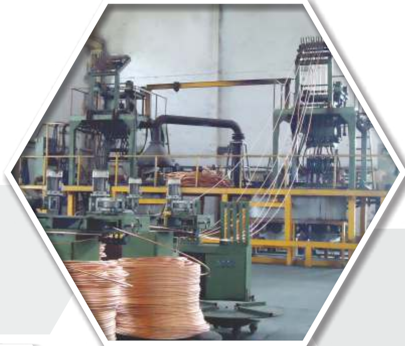
Upcast continuous casting technology
